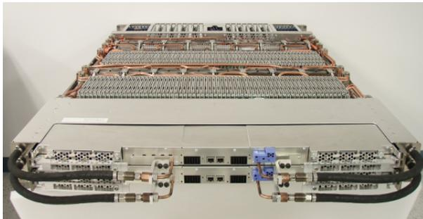
A single node is called an octant (there are eight nodes in one drawer) or a QCM - Quad Chip Module. A QCM contains 4 Power7 chips that are connected in a ceramic module, which gives a 32-way SMP node. The total memory bandwidth of a QCM is 512 GB/s.
