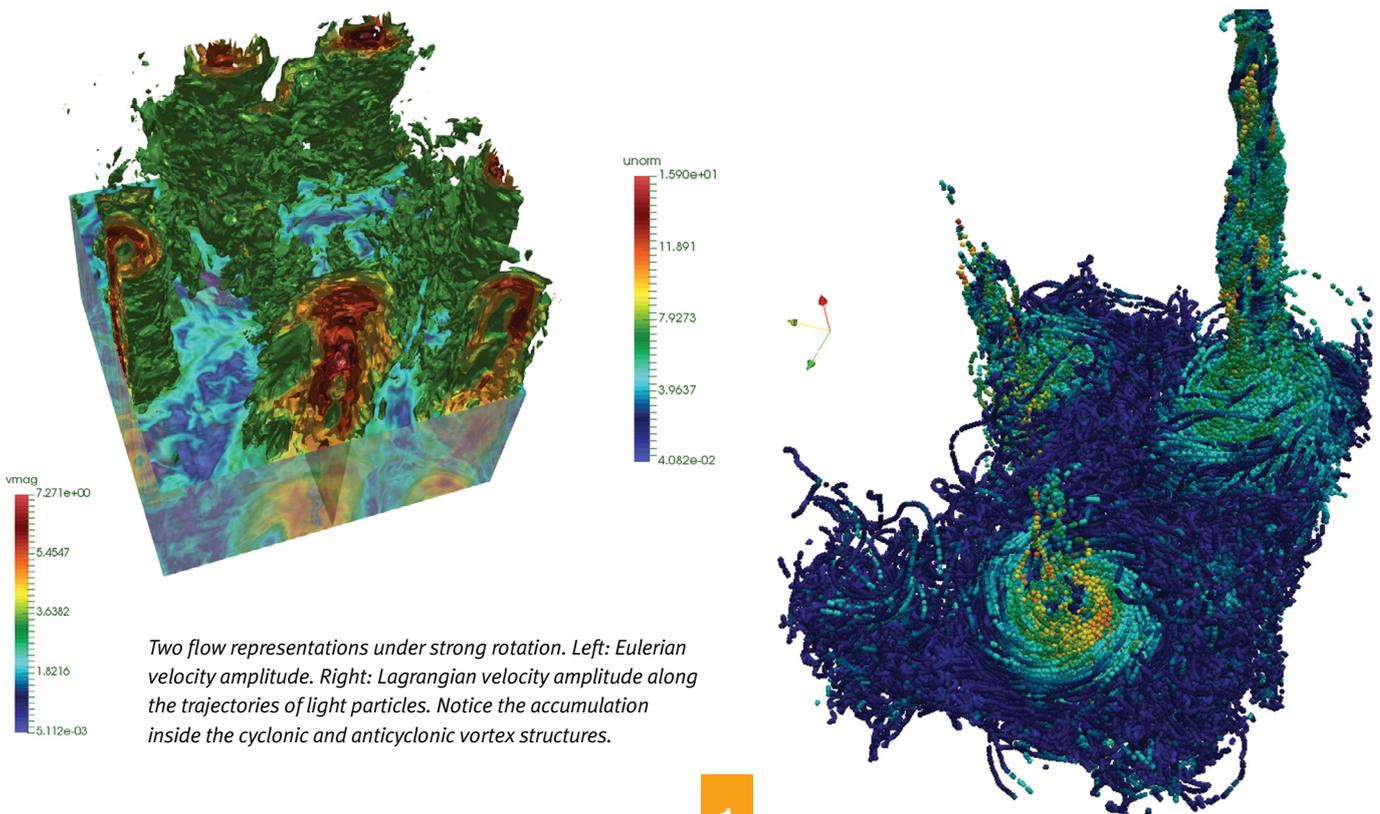
Two flow representations under strong rotation. Left: Eulerian velocity amplitude. Right: Lagrangian velocity amplitude along the trajectories of light particles. Notice the accumulation inside the cyclonic and anticyclonic vortex structures.
