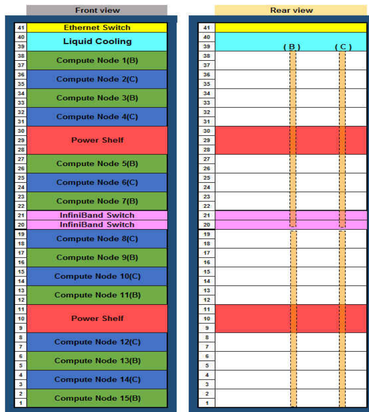
Figure 6: Layout of a D.A.V.I.D.E. rack in the final configuration.
