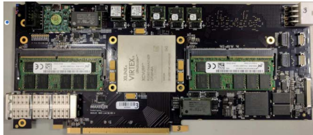
Figure 7: A Maxeler M5C card
