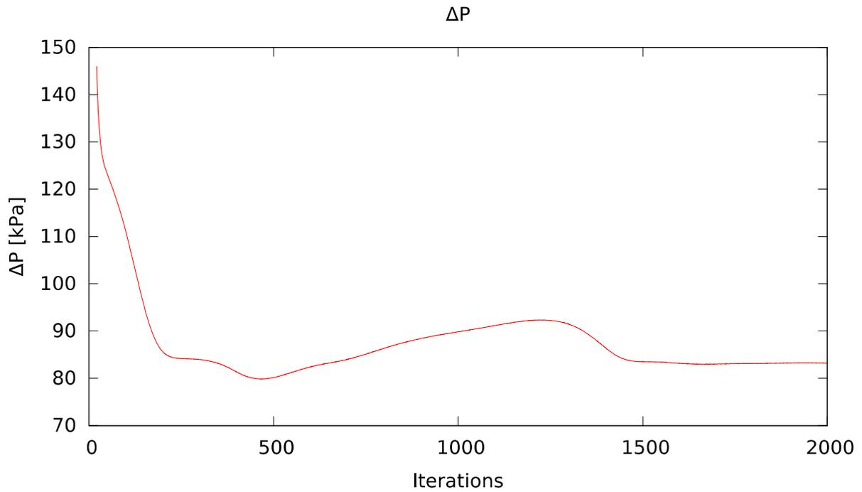
Figure 4 Quantitative monitor of pressure to check physical convergence
