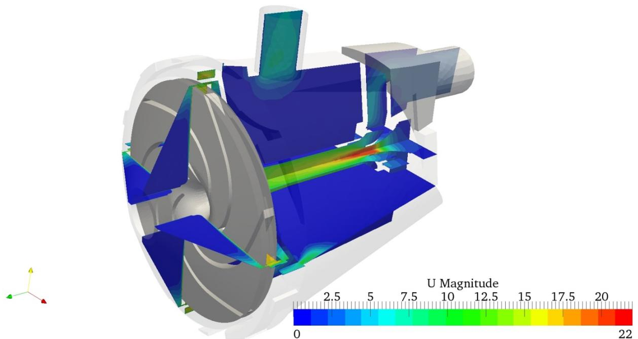
Figure 1 A schematic representation of a centrifugal pump mesh and CFD results.
