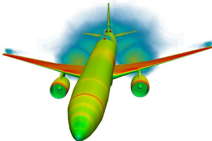
Figure 8: Visualized turbulence wake
