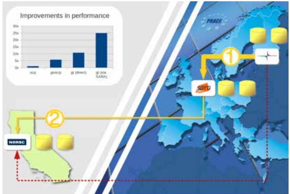
Fig.1. Instead of using a direct but slow connection (dashed red line) between CSC and NERSC, gtransfer (gt) reroutes the data transfer over SARA (yellow lines) and even so achieves a higher performance.
