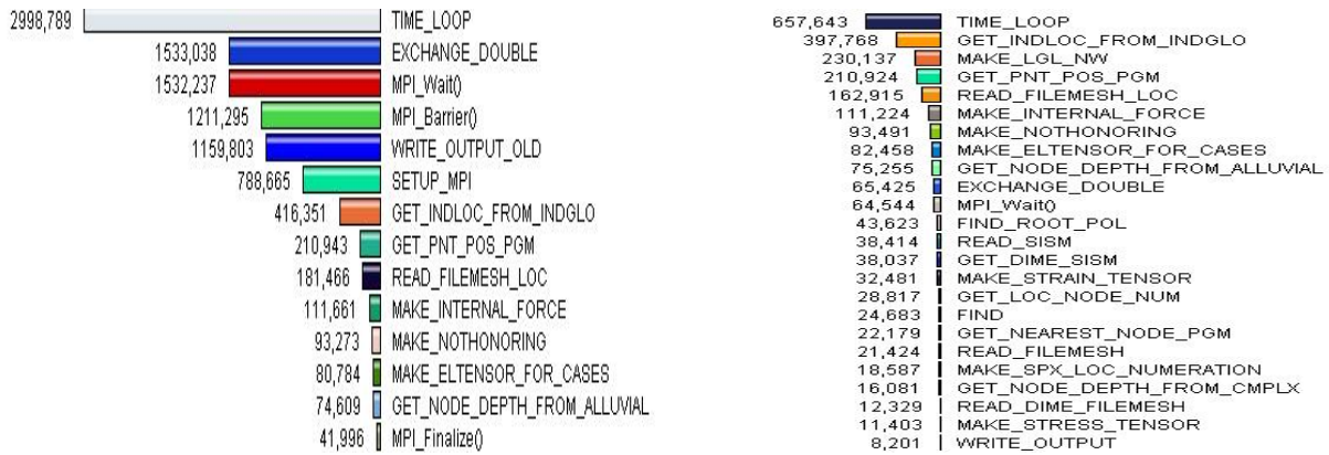
Fig. 4. SPEED, optimization of the I/O and computing phase. Times are in seconds. Old routine on the left “WRITE_OUTPUT_OLD”, new routine on the right “WRITE_OUTPUT”. Old “TIME_LOOP” routine on the left, new “TIME_LOOP” routine on the right.
